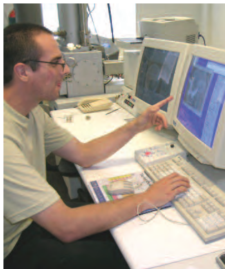
Figure 20 Phil Parkes using a scanning electron microscope with energy dispersive x-ray analysis at Cardiff University to determine the elemental composition of heritage materials undergoing treatment by BSc Conservation students. The SEM was purchased by the University with part funding from the National Museum of Wales under the Joint Research Equipment Initiative (JREI). Its use is shared between these two organisations. Photo: David Watkinson
